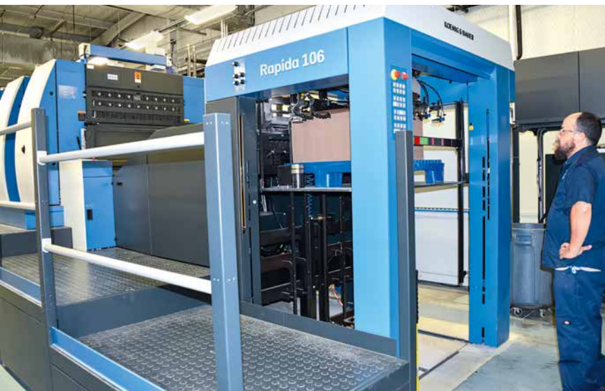
The raised Rapida 106 is fitted with nonstop automatic facilities at the feeder
