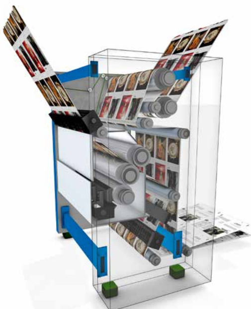
New UV coating unit for the Koenig & Bauer C16
