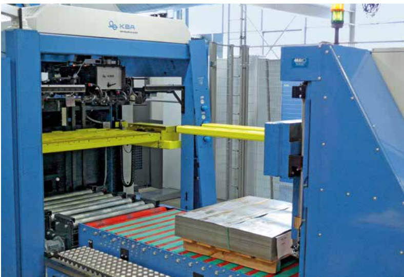
MetalStar 3 automatic pallet changer
