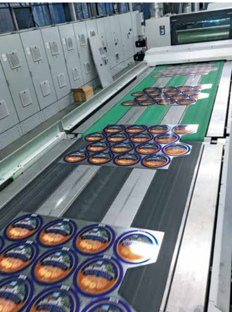
Material savings have the highest priority in metal printing. Here scroll-cut sheets are printed and coated. These panels are punched out to make optimum use of the substrate
