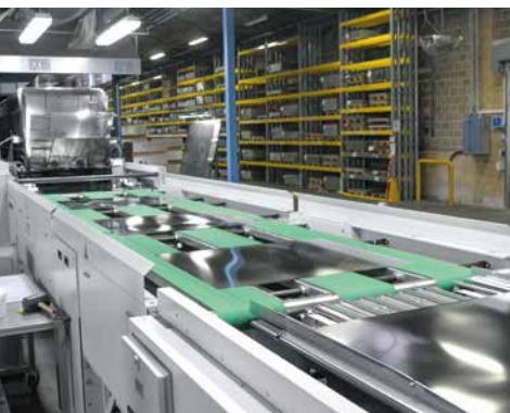
On the coating dwell section the coating applied has time to spread on the sheet, which prevents unwanted structures
