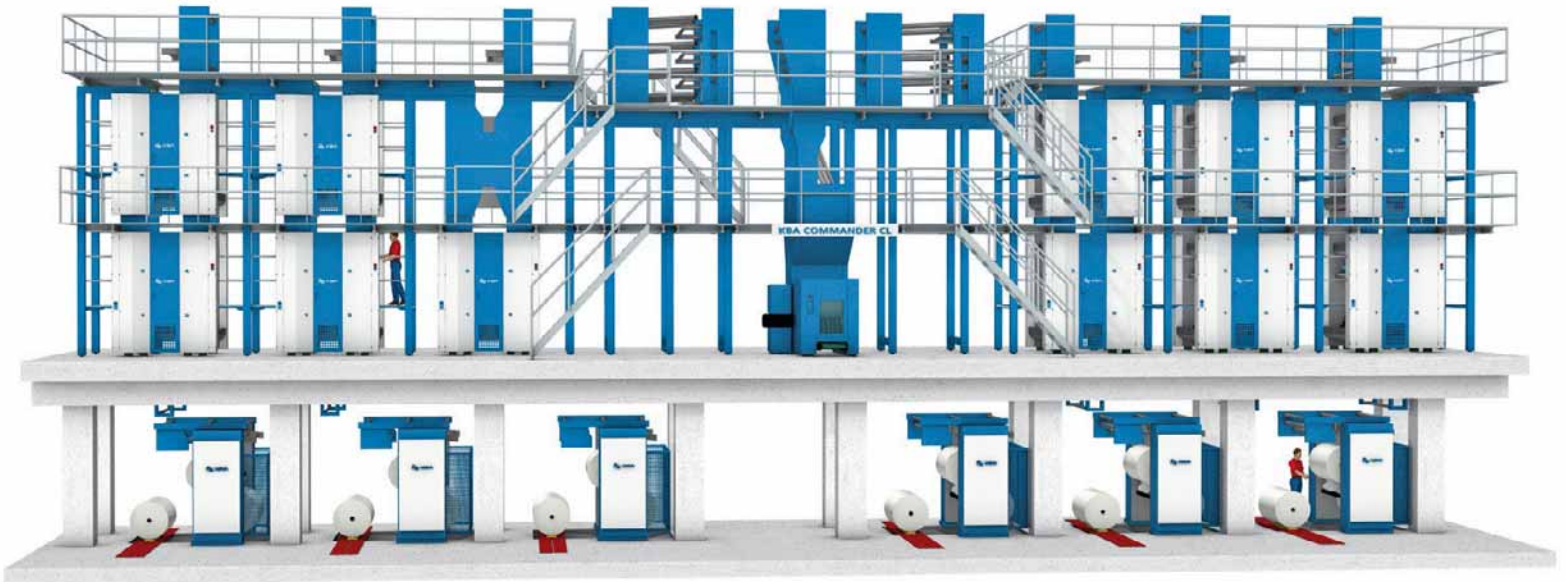
Above: The second Commander CL 4/1 consists of five four-high towers for 4/4 printing, a 1/1 printing unit, a KF 5 jaw folder with a ribbon stitcher and six Pastomat reelstands
