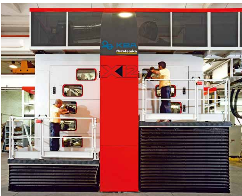
Changing sleeves on the high-tech EVO XG 12
