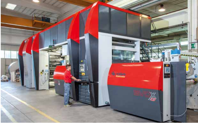
Left: the EVO XG series is engineered for larger printing widths of up to 2m (6.5ft) and high speeds of up to 600mpm (1,825fpm)
