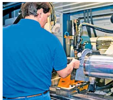
Close cooperation with the parent KBA in Würzburg: measuring, replacing, grinding of the bearer rings
