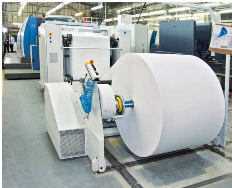
The firm's existing six-colour Rapida 106 installed in 2010 was retrofitted with roll-to-sheet kit
