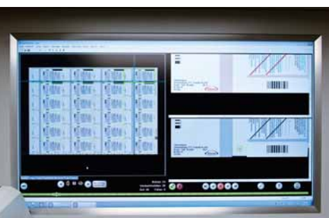
QualiTronic PDF compares every sheet and blank electronically with the customer's PDF data. Even the smallest print errors are detected
