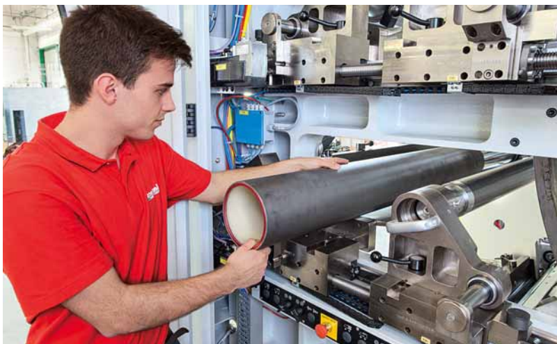
Ergonomic sleeve changing on the gearless EVO XD
