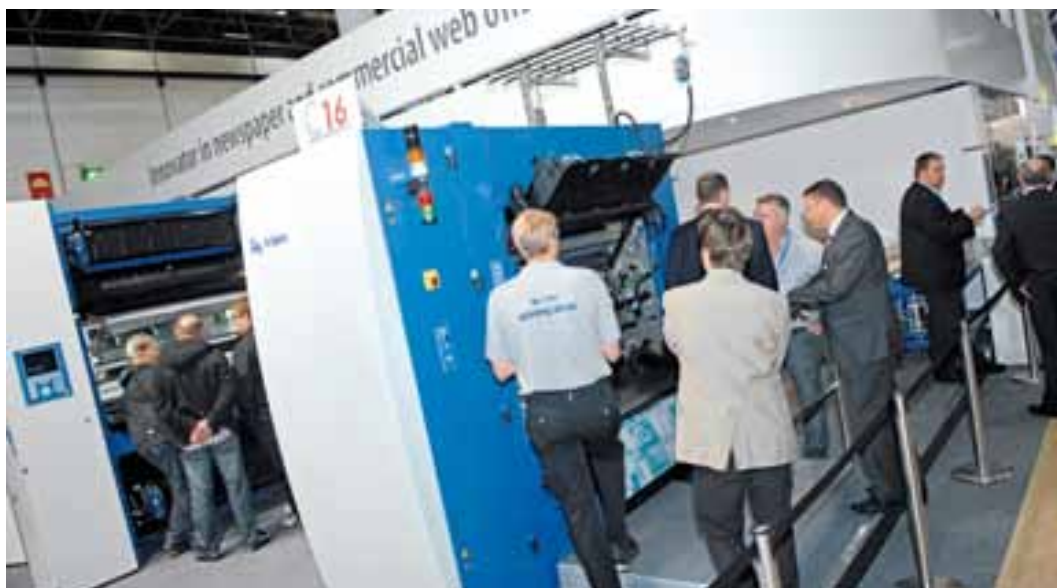
A C16 printing unit at Drupa demonstrated high-speed automatic plate changing in less than sixty seconds
