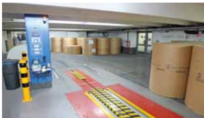
The weighing station in the reel store is part of the KBA Patras A automated reel-logistics system
