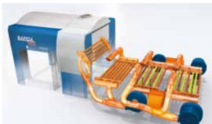
Reutilising the air circulated in the dryer can substantially reduce the amount of energy consumed by KBA VariDry BLUE dryers compared to conventional infrared/hot-air dryers
