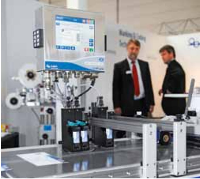
KBA-Metronic exhibited its new udaFORMAXX separator with betaJET thermal inkjet technology for printing folding cartons, packaging blanks etc
