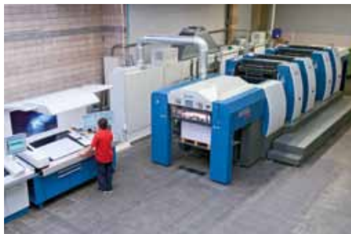
The two five-colour Rapidas were joined by a perfector version for two-backing-two
