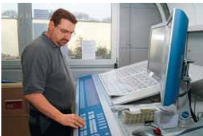
When printing labels it is handy to have all the operational data stored at the console for repeat jobs, so that manual settings are rarely needed even at the feeder and delivery
