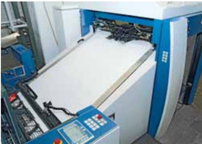
The Rapida 106 at ak-medien has a DriveTronic SIS sidelay-free infeed
