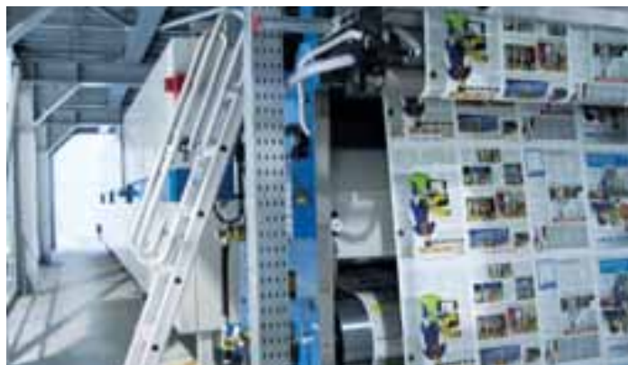
A semi-coated web leaving one of the four heatset dryers will subsequently be gathered with coldset newsprint webs in the folder superstructure
