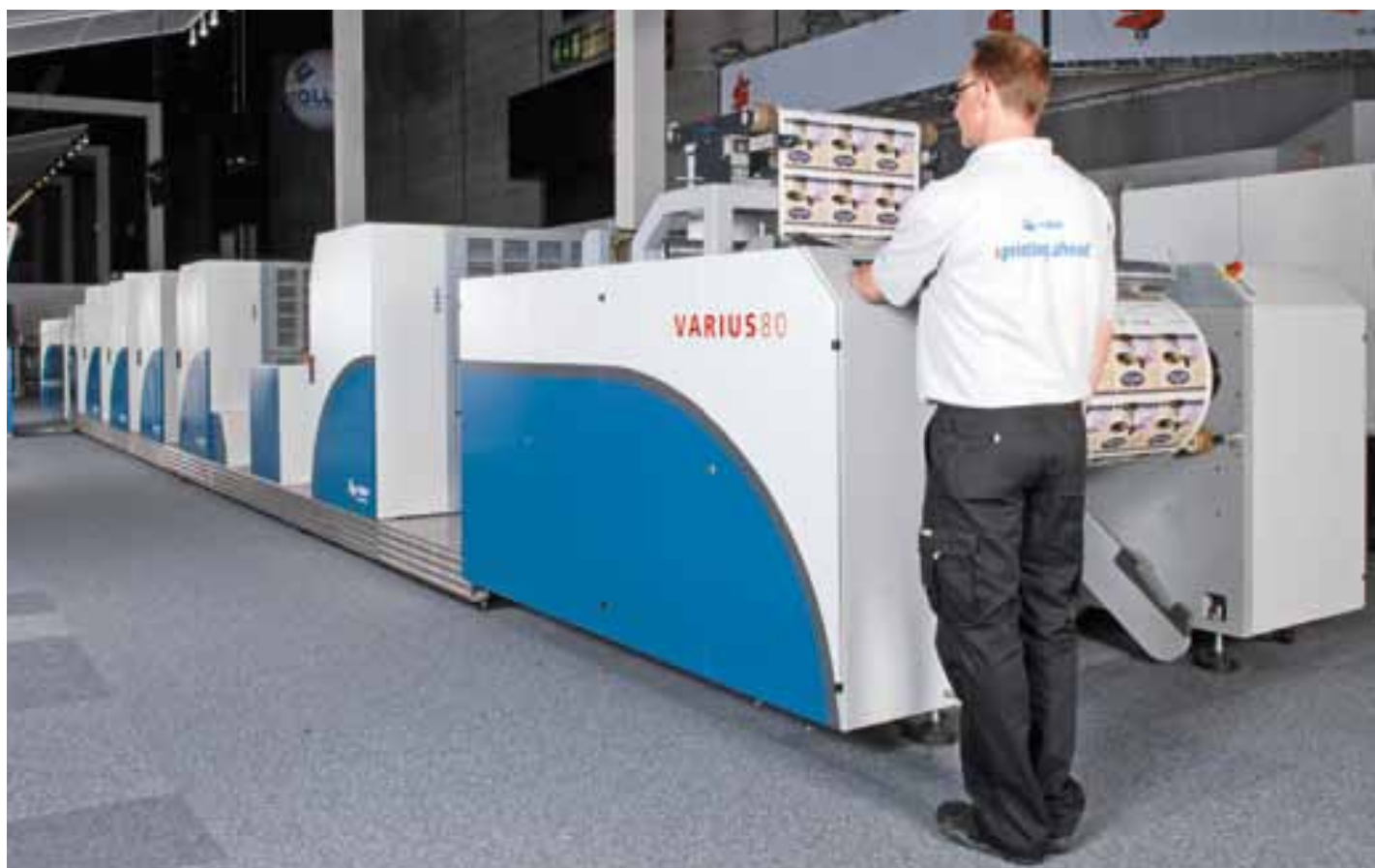
The Varius 80 has a maximum web width of 800mm, a maximum rated production speed of 400 metres per minute, can handle substrates 30µm to 800µm thick and can deliver image formats 21 to 34 inches long
