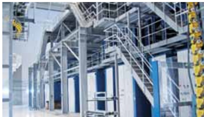
One of the three press sections comprising four compact towers with an overhead thermal dryer above each of the two outer sections
