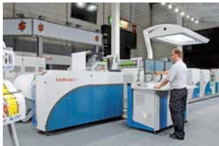
A new approach: KBA-MePrint's variable-format UV web offset press, the Varius 80, targets the high-growth market for flexible packaging by delivering fast job changes, a superior print quality, low waste levels and short-run economy
