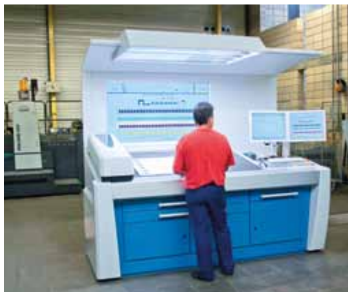
All three Rapidas are controlled from new-style ErgoTronic consoles featuring a wall screen, an ACR (automatic camera register) system and inline KBA QualiTronic colour control
