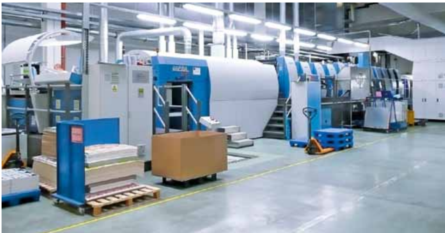
The new Rapida 106 at Model Obaly boasts an array of automation and finishing components that includes the Vinfoil cold-foil module in the background
