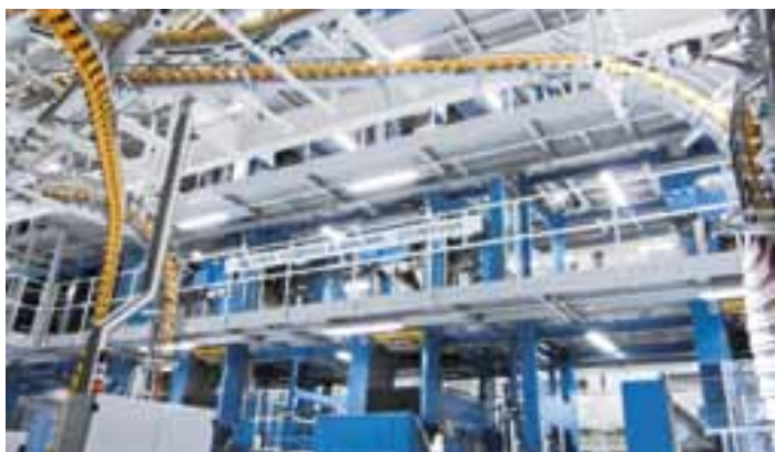
Three folders with copy transport systems are located in the centre of the Cortina press line
