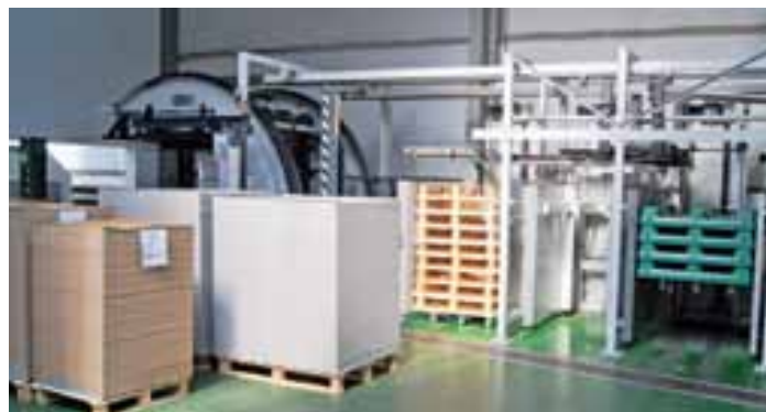
A pile turner is used to transfer blank substrates from the transport system to the infeed pallets
