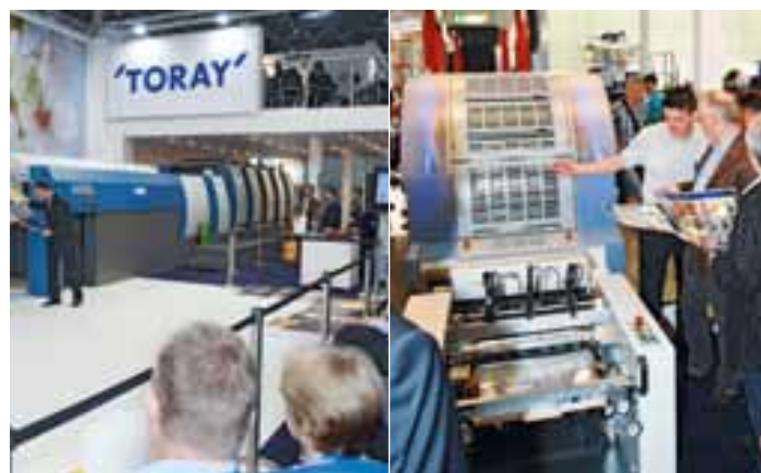
Green printing: two KBA presses – a waterless Genius 52UV and a dampener-free Rapida 106 five-colour with UV coater – on the adjacent Toray stand demonstrated quality excellence on an array of challenging substrates
