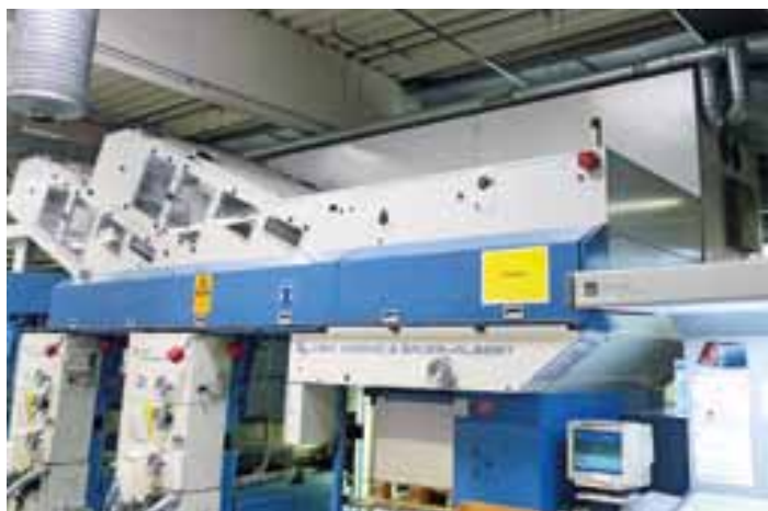
The KBA Rembrandt 104 two-colour sheetfed gravure press commissioned in 1994, with its characteristic drying section
