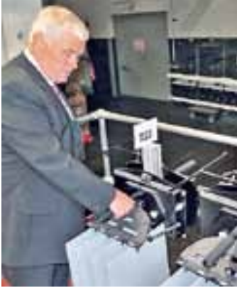
BNN decided not to install a plate transport system right up to the printing couples, instead opting for carriers holding sets of sorted plates, as demonstrated here by plant manager Georg Siepman
