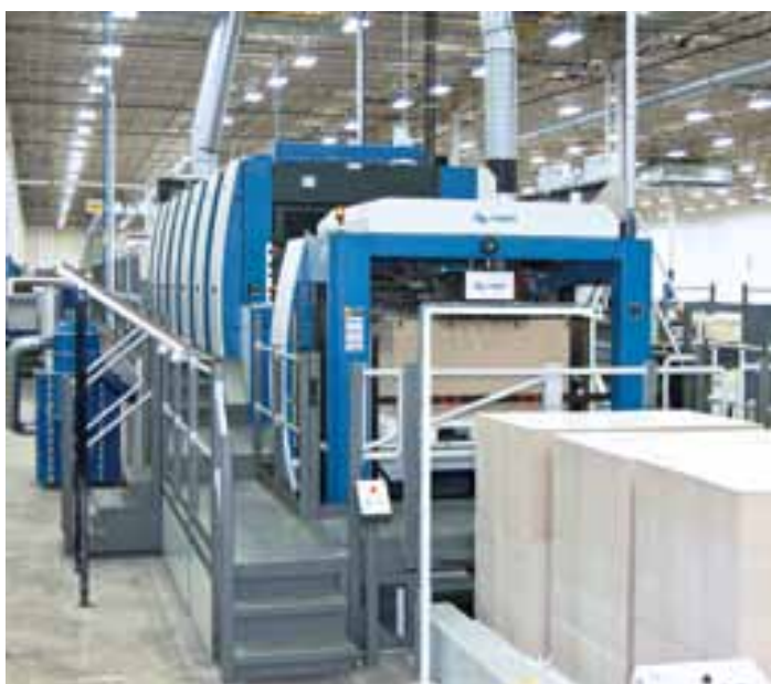
The Rapida 145 at WG Anderson is embedded in an automated pile-logistics system
