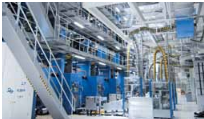
Configured with twelve towers and reelstands, three folders and four thermal dryers, the big Cortina press line is not only an imposing sight but also impresses visitors to the production plant with the superb quality of the copies it delivers
