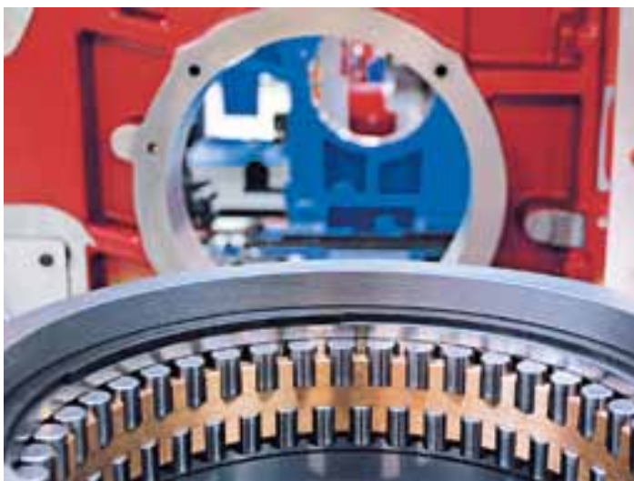
Zero-play antifriction bearings, which have long been a standard fitting in Rapida presses, also help reduce energy consumption
