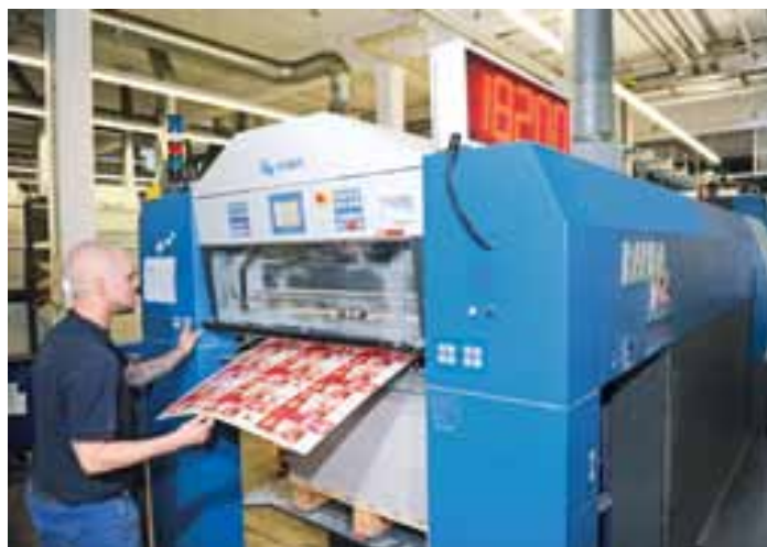
Press operator Toni Tomm has complete control of the new Rapida 106, which can print some substrates at its maximum rated output of 20,000sph but usually runs at around 18,000sph
