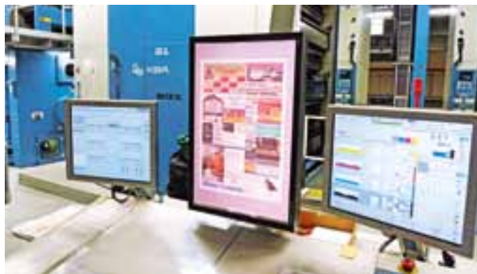
One of three ErgoTronic consoles for the Commander CT: on the left the screen for monitoring registration, in the centre the soft-proof monitor, on the right the touch screen for press operation
