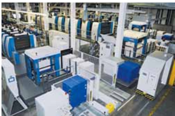
Colorpack's modern press room houses two medium- and two large-format Rapidas, all embedded in an automated substrate logistics system
