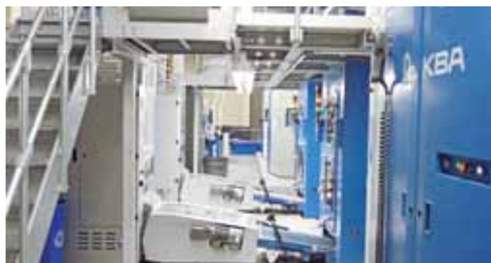
The two folders and transfer stations at the Ferag conveyor are located centrally between the four towers
