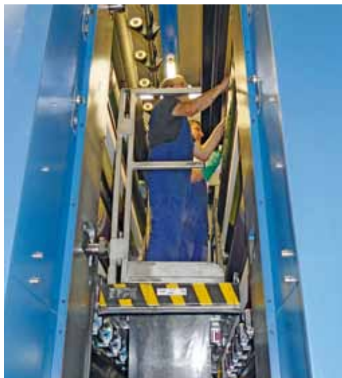
BNN press operators like the easy access via lifts to the slide-apart printing couples
