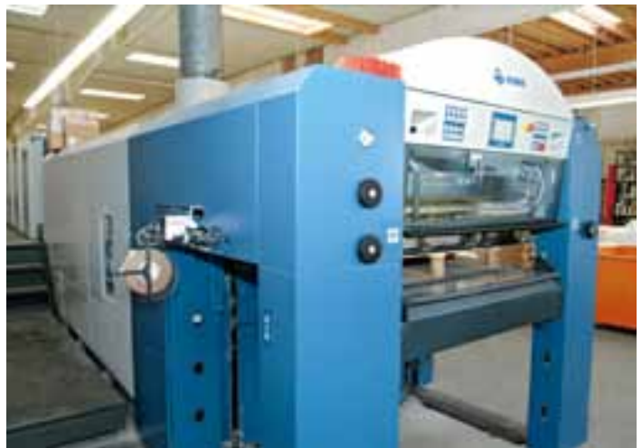
A tag inserter ensures that after being inspected by the QualiTronic ColorControl software flawed items can be separated from saleable items
