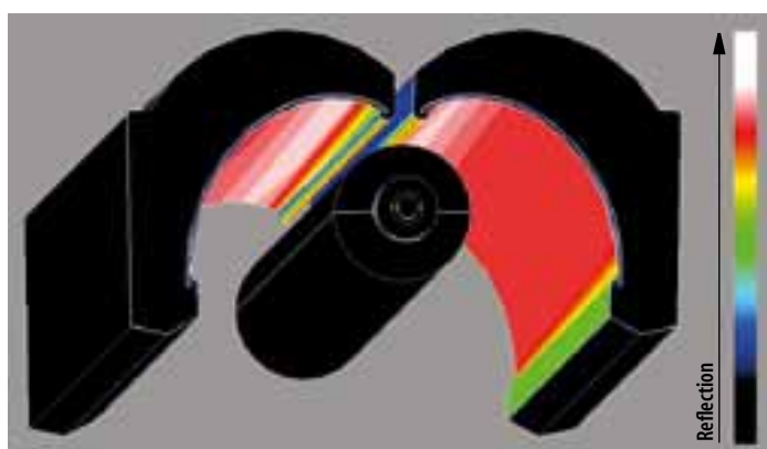
An optimised reflector geometry and better heat management at the radiators improve energy efficiency when drying
