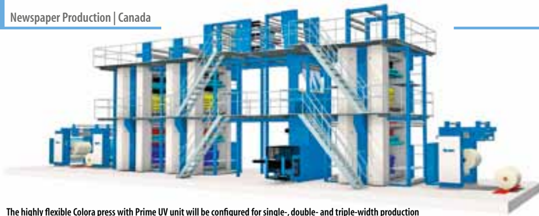
The highly flexible Colora press with Prime UV unit will be configured for single-, double- and triple-width production
