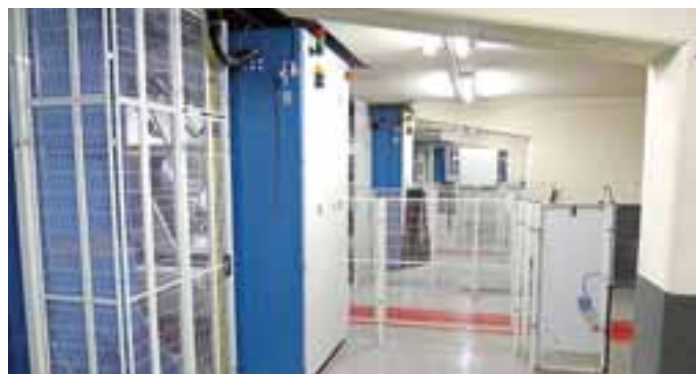
The reelstands, which because of the sheer size of the triple-wide reels and cores had to be fitted with protective screens, also fitted neatly in the existing hall
