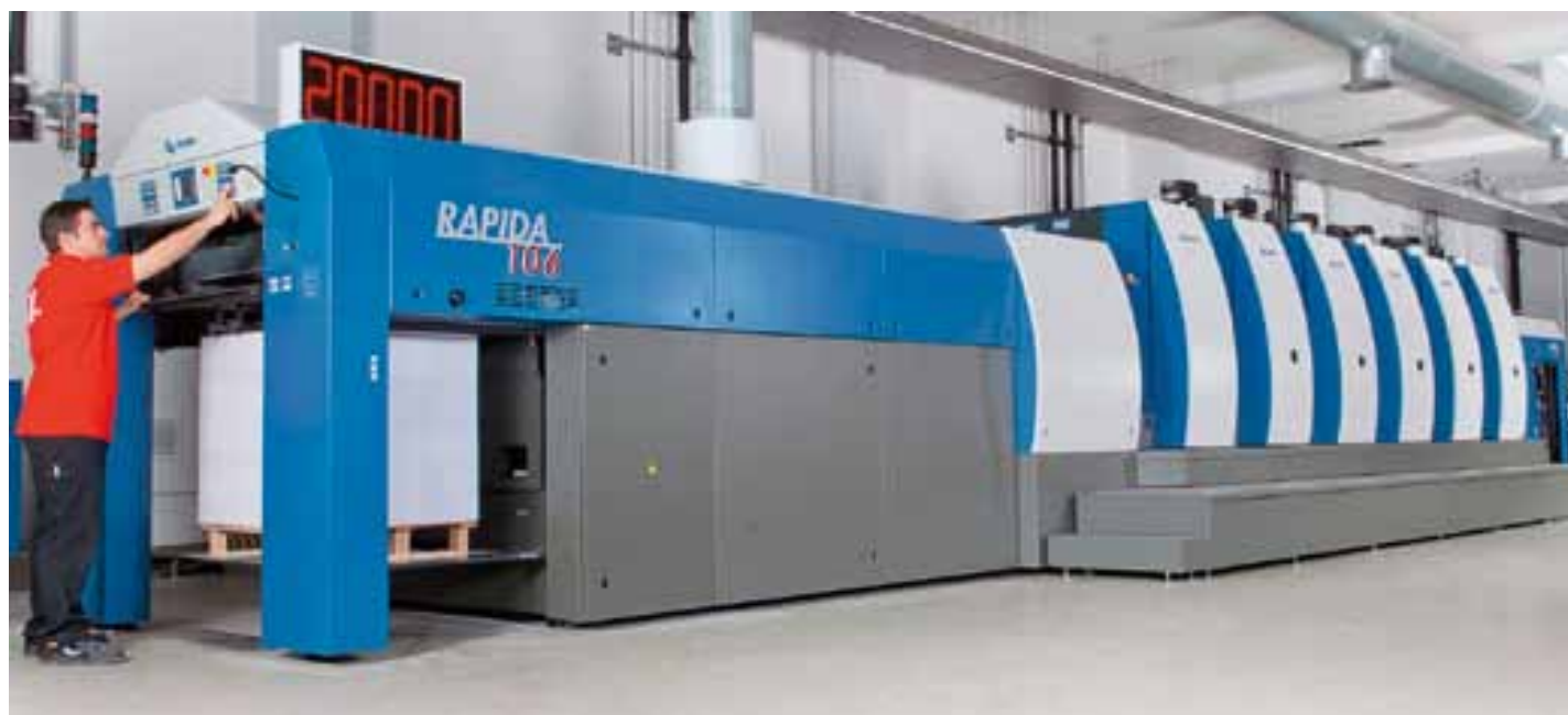
A five-colour medium-format Rapida 106 with aqueous coater came on stream at ADV Schoder's Gersthofen plant in August
