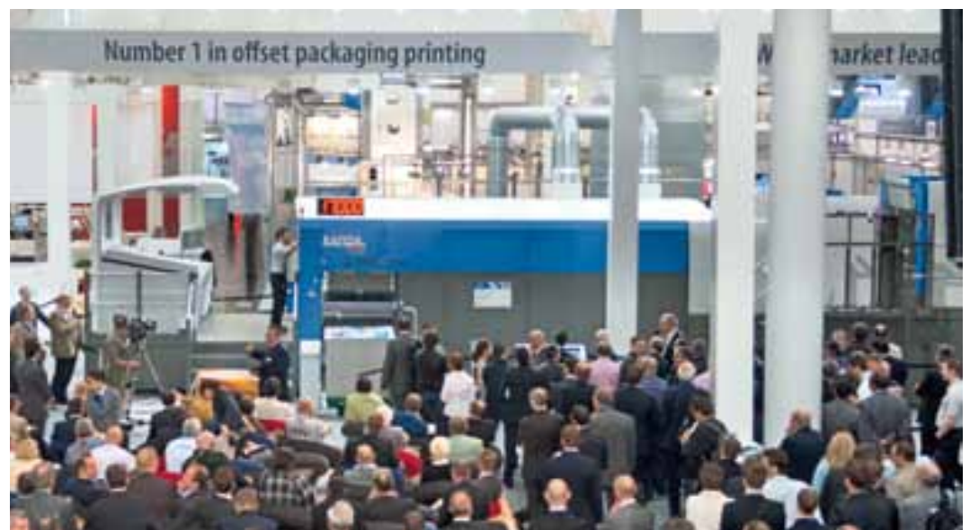
Litho high-spot: our new Rapida 145 was the largest sheetfed press at the show, attracting big audiences for demonstrations of straight printing at 17,000sph and 4/4 perfecting at 15,000sph – a capability that is unparalleled in this format class, as is automatic plate changing with DriveTronic SPC in just over sixty seconds and a complete job change in just a few minutes
