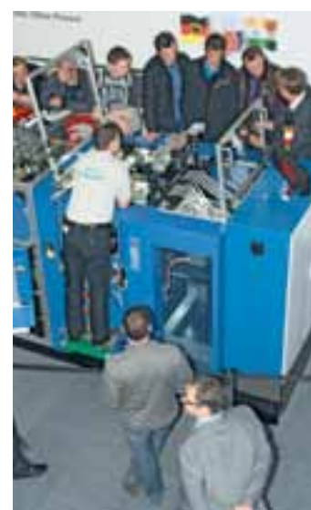
The C16's new quarterfold with low-maintenance belt tensioning for speeds of up to 65,000iph was a major draw for web offset printers
