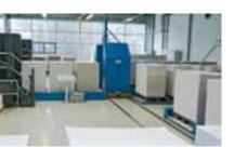
The automated pile-logistics system for the three large-format Rapidas includes a shuttle trolley that conveys the prepared piles to buffer stations at the feeders
