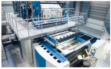
Ultra-fast edition changes thanks to convenient lifts that provide optimum access to printing couples and PlateTronic automated on-the-fly plate changers
