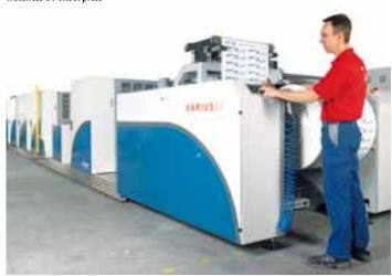
KBA-Metronic's udaFORMAXX separating system for folding cartons has an integrated, freely programmable betaJET thermal inkjet unit for addressing, offline coding etc
