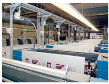
The eight-colour Rapida 106 is connected to an automatic ink-pumping system, but the six-colour (in the background) is not because it is often used for special colours
