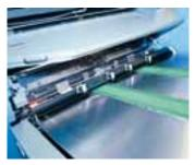
The feeder board for the Rapida 145 has just two suction belts and the proven DriveTronic SIS sidelay-free infeed adopted from the Rapida 106
