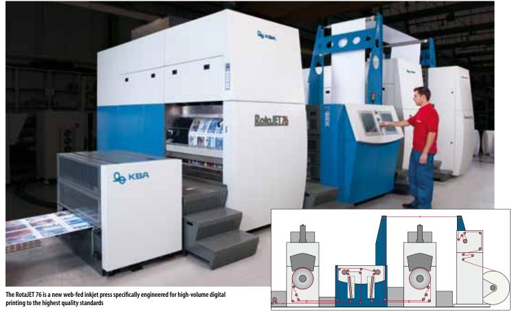
The RotaJET's ingeniously simple web leads promote a precise web tension and allowed the length of the press to be reduced substantially compared to other installations
