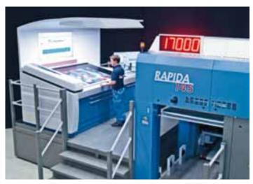
View across the new Rapida 145's overhead venturi delivery to the new ErgoTronic console with integrated measurement and control systems
