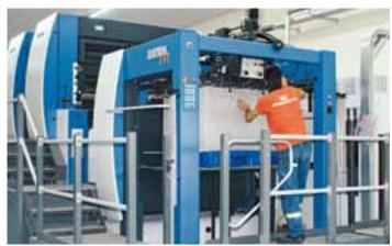
The large-format Rapida which came on stream in March 2011 is mounted on a plinth to accommodate the higher piles common in board printing
