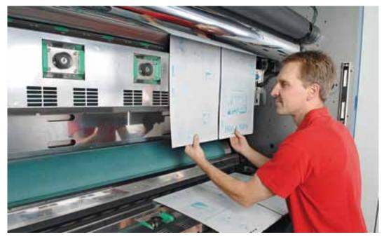
The Commander CL can be fitted with optional automatic or semi-automatic (pictured here) plate changers
