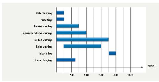
Makeready diagram for a large-format Rapida with all options, showing how simultaneous sequences can cut makeready time (non-binding example)
