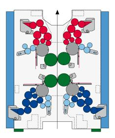
The printing units in our new Commander CL are just 2.75m high, easily accessible and precision-engineered to deliver a superb print quality
