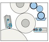
CleanTronic Synchro in operation: Left: simultaneous blanket and cylinder washing Right: blanket washing by two bars simultaneously
