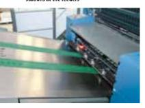
The elimination of rollers and brushes at the feeder board is a neat solution; the red light is emitted by the DriveTronic SIS sidelay-free infeed system
