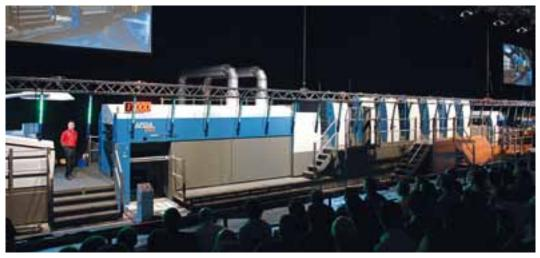
With a maximum output of 17,000sph in straight mode and 15,000sph in eight-colour perfecting, our new, fully automated Rapida 145 is not only the makeready world champion but also the absolute speed champion in large format
