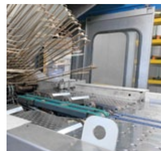
Venturi air-nozzles for reliable sheet transportation with minimum contact
