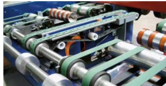
Tapes with larger contact surface for heavy sheets
