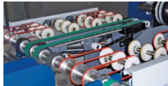
Belts with less contact surface for light sheets
