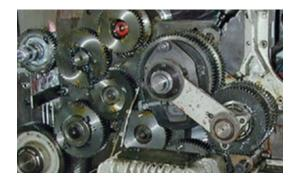
The conventional mechanical coupling has a complicated and irregular slip adjustment system and the drive gears are subject to wear due to high loads. The pneumatic friction clutch replaces the rigid mechanical coupling that links the main gear with the counter pressure cylinder and the coating cylinder.
