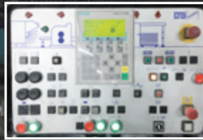
Control panel on the coating machine
