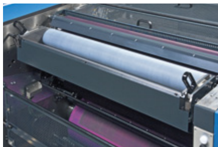
Ink duct with ceramic-coated roller
