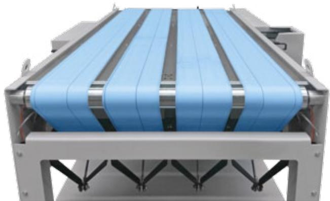
are deployed. This feature not only ensures a steadily uniform belt tension, but also a constant distance from the belt shaft to the preceding station. The result: a significantly improved reliability of the production process. Finally, the new conveyor belts can be fastened easily by a spiral fastener. This means no more cumbersome gluing of belts and a reduction in make-ready times by up to 85 %.
