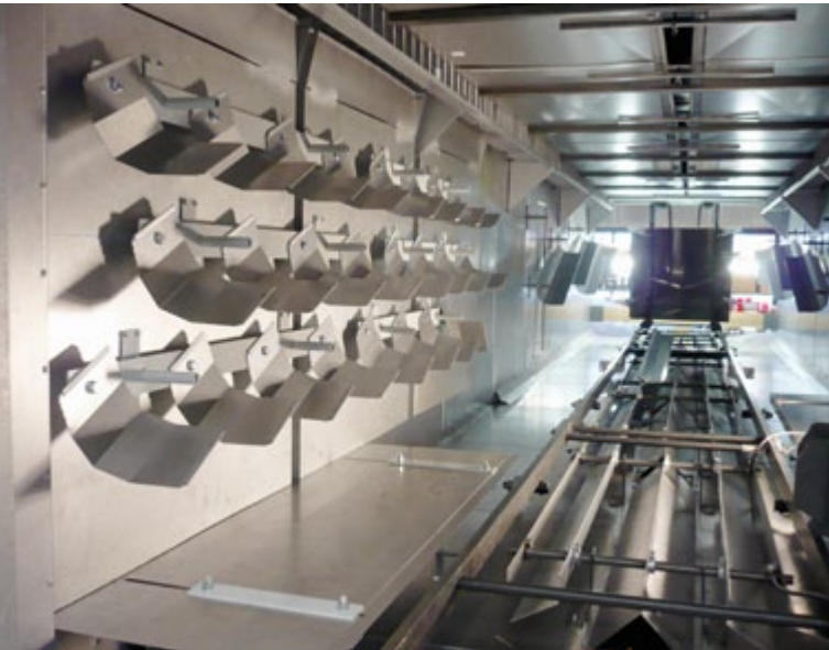
AirFlow Pro with special baffles laterally – for highest quality demands, with double-walled version
