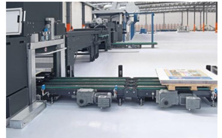
Two bridge conveyors for connecting two production lines by bridging stacker (upstream line) and feeder (downstream line)
