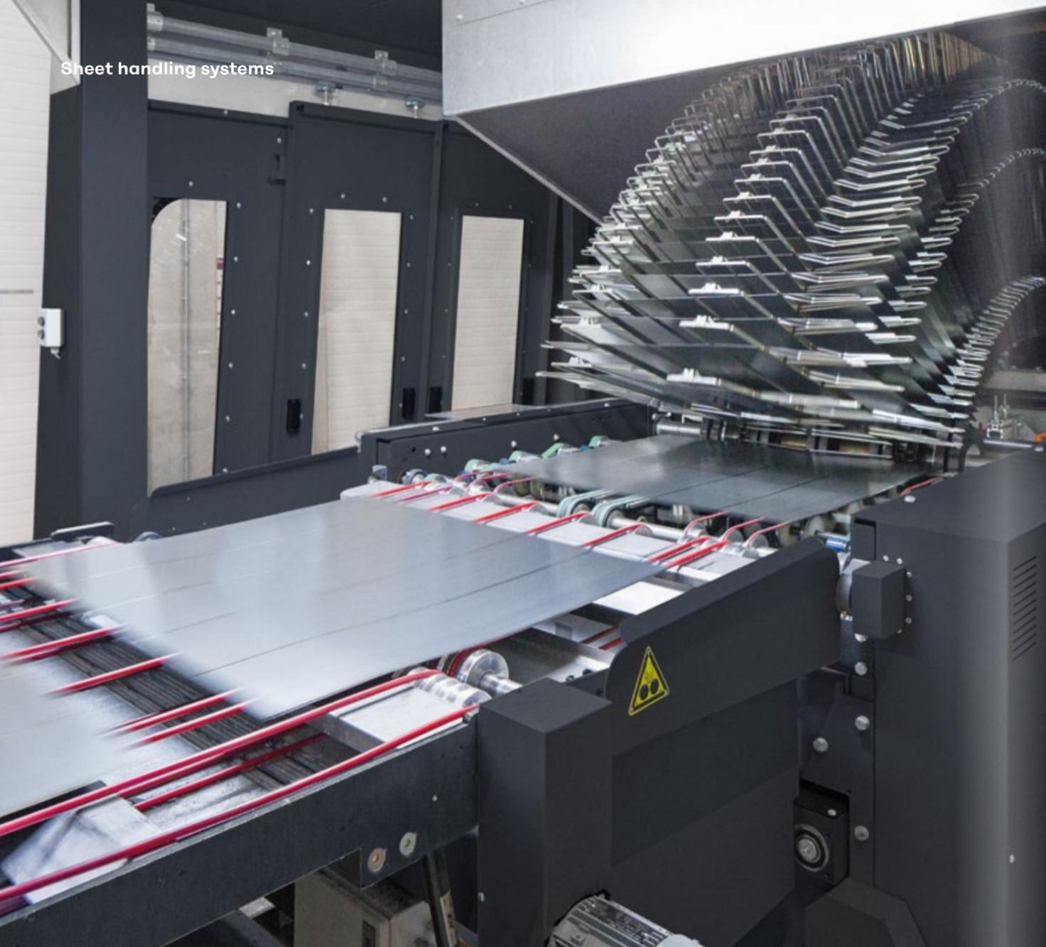
Round belt transportation bridge and dynamic sheet control for loading machines.
