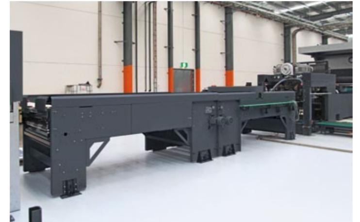
Bridge conveyor with additional front edge alignment in combination with an intermediate feeder (viewed from the drive side with second bridge conveyor following)
