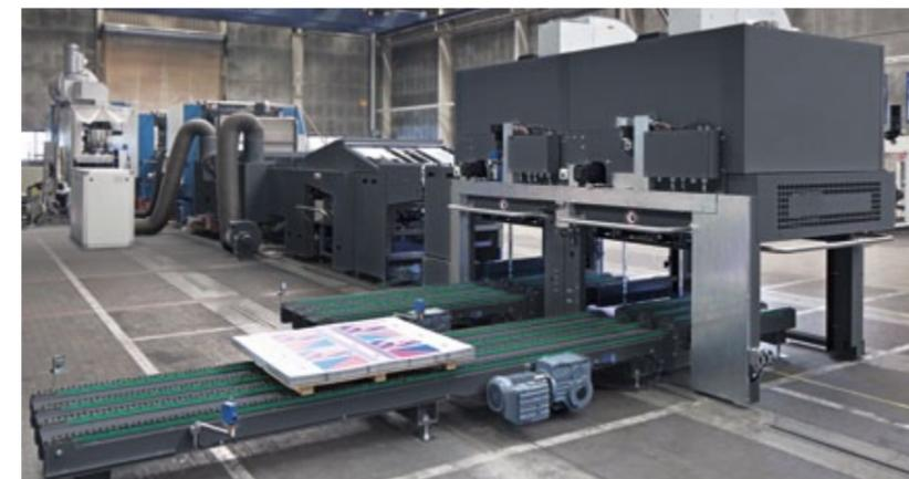
Optional stack removal via a side chain conveyor
