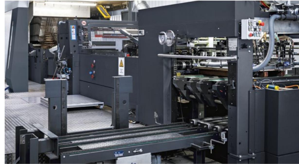
Side chain conveyor for feeder 780
