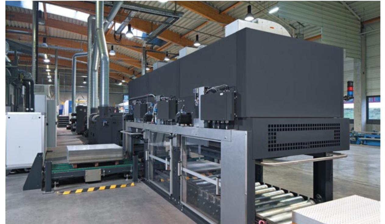
Triple-box stacking including waste sheet stacking and side chain conveyor
