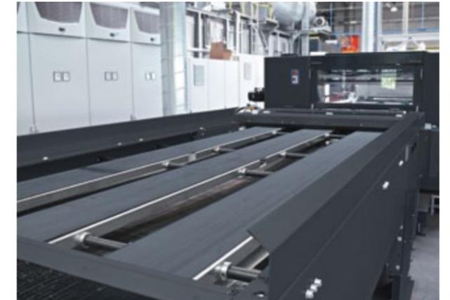
Sheet transport after a UV backside dryer
