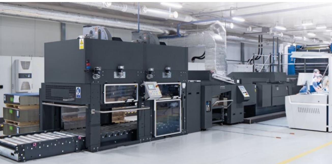
Double-box stacking unit in a MetalStar 3 printing line
