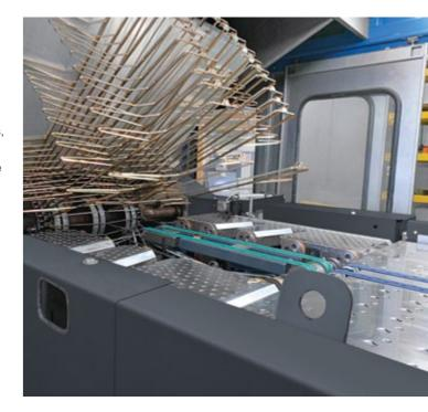
$\label{lem:control} \textbf{Venturi transport and loading machine with dynamic sheet control}$
