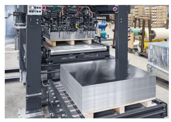
Option: Stop&Turn with laser-assisted pile centring
