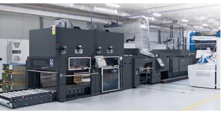
Double-box stacking unit in a MetalStar 3 printing line
