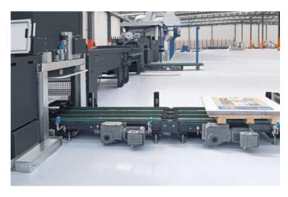
Two bridge conveyors for connecting two production lines by bridging stacker (upstream line) and feeder (downstream line)
