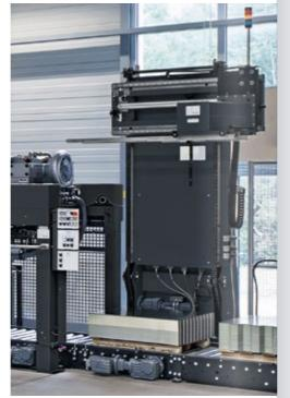
Semi-automatic pallet changer, type 775 for feeder 780 on coating lines
