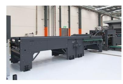
Bridge conveyor with additional front edge alignment in combination with an intermediate feeder (viewed from the drive side with second bridge conveyor following)
