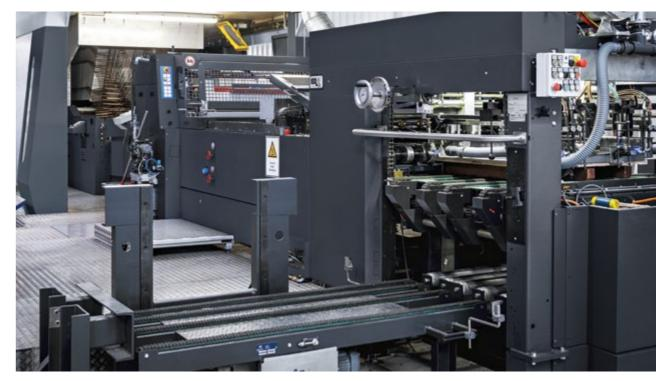
Side chain conveyor for feeder 780
