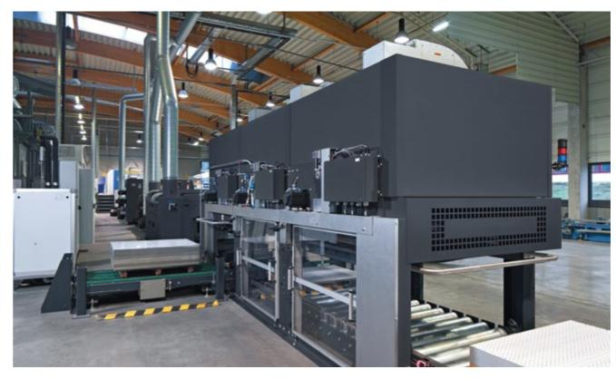
Triple-box stacking including waste sheet stacking and side chain conveyor
