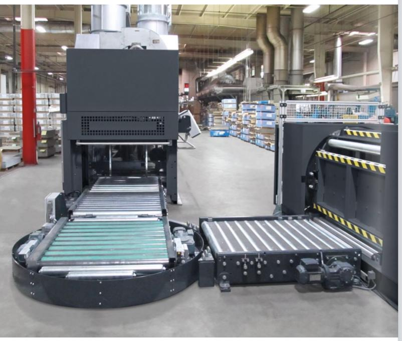
Roller conveyor with turntable and inline pile turner type 821
