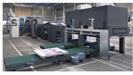
Optional stack removal via a side chain conveyor
