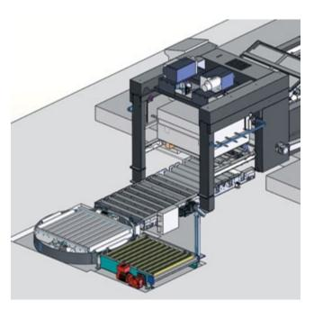
Roller conveyor with turntable for feeder type 780
