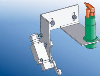
**Contact-free overpiling switch on the feeder** For MetalStar 2 The overshoot detector monitors the gap between the previous and the following sheet by means of a photo sensor on the feeder table. If this gap is not detected, this is recognised by the sensor as an early sheet, and the press stops with a fast stop.
