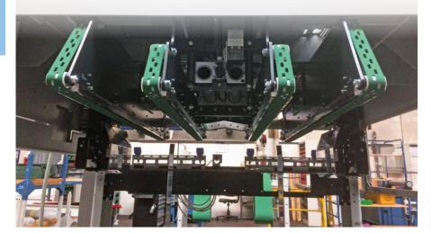
VacStack vacuum-operated overhead brake For LTG single stacker
