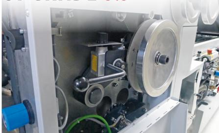
The fine adjustment of the circumferential register serves to position the transverse recess of the coating cylinder exactly. The two friction discs are replaced by two toothed adjustment wheels. This eliminates the slip, and exact positioning of the coating cylinder, down to 0.1 mm, is possible straight away. There is no further need for any repeated, time-consuming corrections.
