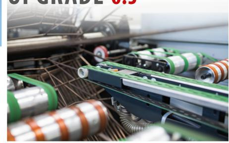
Dynamic sheet accelerator For LTG unloading machines
