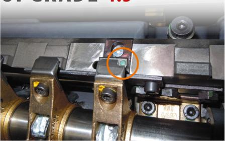
**Gripper edge sensors** For all Sprint multi-colour printing machines Sheet detection, irrespective of material and surface, is achieved by way of two inductive sensors. The stable sensor response serves to significantly enhance process reliability. The insensitivity towards dirt and simple cleaning ensure constant sheet travel and thus maximum productivity. Straightforward positioning and fast replacement permit considerable shortening of the press downtime.
