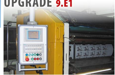
Modern control and drive system For LTG Mailänder printing and coating lines
