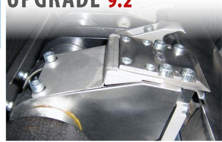
Motor-driven diagonal register For Mailänder printing presses types 122A and 222
