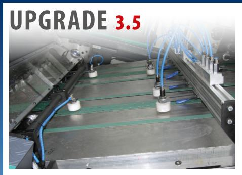
**Feeder sheet separation** For all Sprint multi-colour printing machines The incoming sheet is lifted by a timed air pulse which ensures a smooth, virtually contactfree separation from the following sheet.
