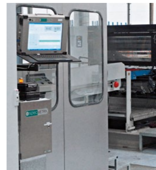
Inline coating thickness measurement system
