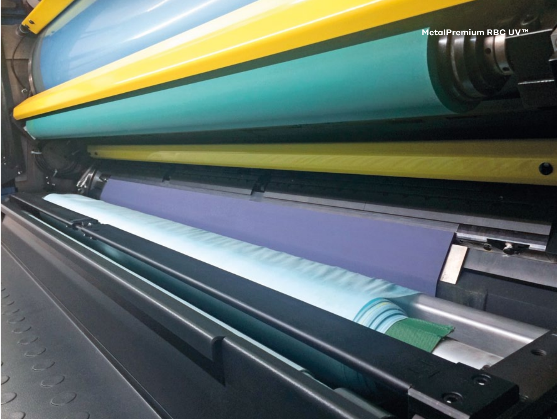
Innovative blanket MetalPremium RBC UV™ based on a film as carrier in the new type of pneumatic blanket clamping and tensioning device
